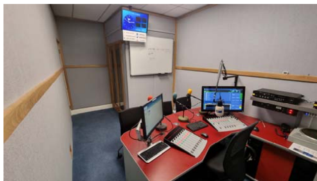
(Left) Studio 1 at Baltic Chambers with the original foam sound-deadening panels and open view of the transmission racks. (Right) the studio following refurbishment in 2022 which saw the installation of industry-standard sound absorption panels with a cloth overlay and boxing-in of the transmission equipment which significantly improved the studio acoustics and reduced the room's temperature.
